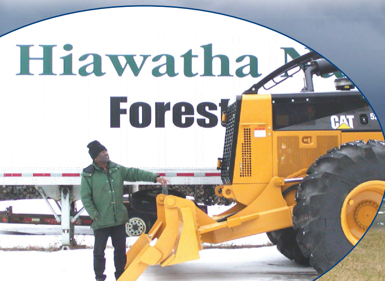
Toby Rhue is proud of their new Caterpillar skidder. He asked for and got the company to send it “green loaded”—so all of the hydraulic fluids were soy biobased from the start—a first for Hiawatha National Forest.
